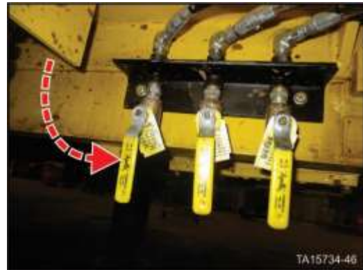
Figure 22. Open air reservoir bleed valves
