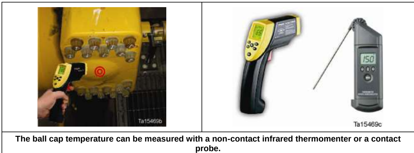
Figure 48. Measuring ball cap temperature
