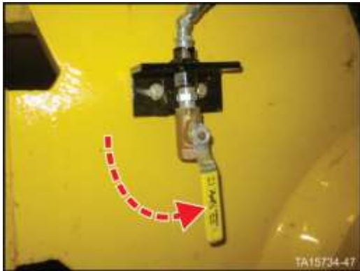
Figure 22. Open air reservoir bleed valves
