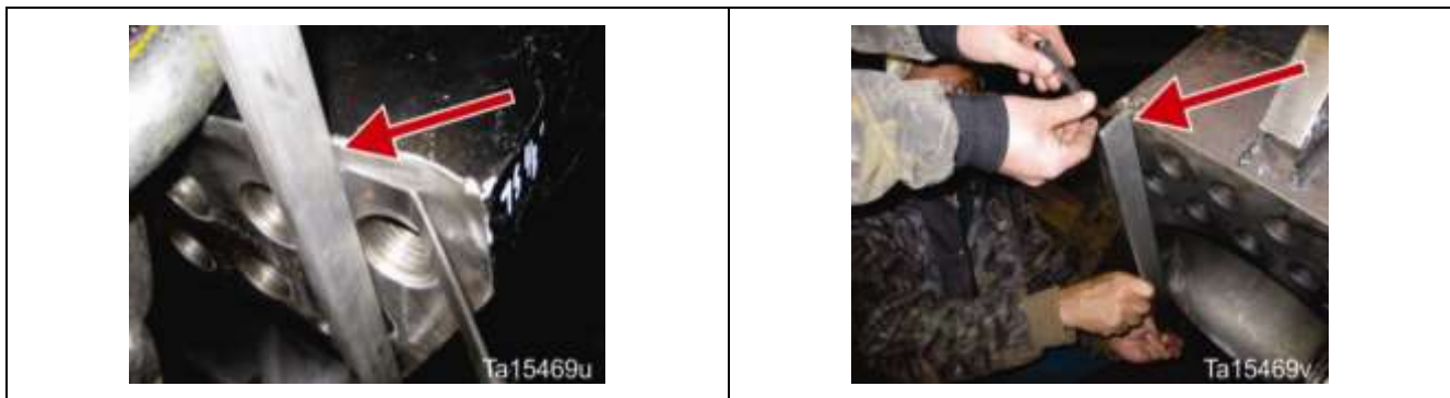
Figure 63. Feeler gauges under straight edge
