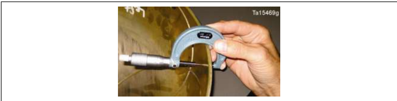
Figure 55. Measure liner thickness with a point micrometer
