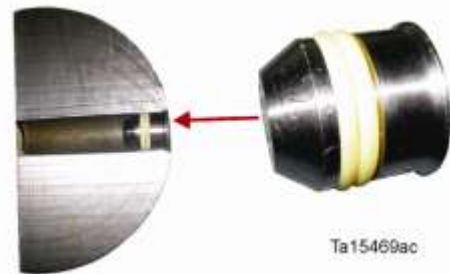
Spherical ball joint greased through cap – hole is plugged (refer to SIL 413)
