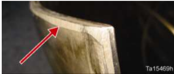
Figure 56. Bronze liner chamfer (bevel)
