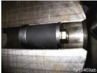
Spherical ball joint greased through cap – hole is plugged (refer to SIL 413)
