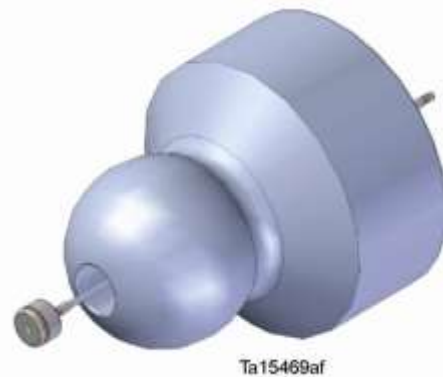
Spherical ball joint greased through ball – hole is plugged and grease hose connects to the plug plate
